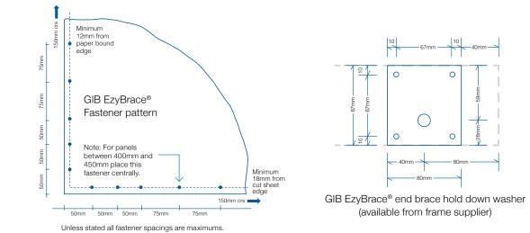
In order for GIB® systems to perform as tested, all components must be installed exactly as prescribed. Substituting components produces an entirely different system and may seriously compromise performance. Follow the specifications. This specification sheet is issued in conjunction with the publication GIB EzyBrace® Systems
