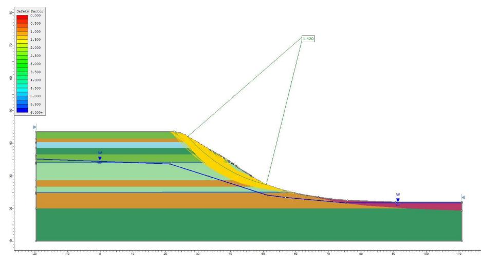
SLIDE 2018 model – Existing Site – Gravity Conditions – FOS required: 1.5
